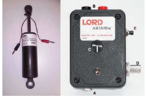
Figure 2. MR damper model RD-8040-1 with current driver by Lord Corporation.
