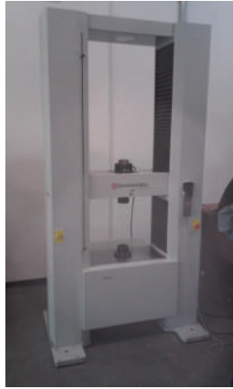
Figure 4. Universal testing machine was the model AG-IC/100kN by Shimadzu.
