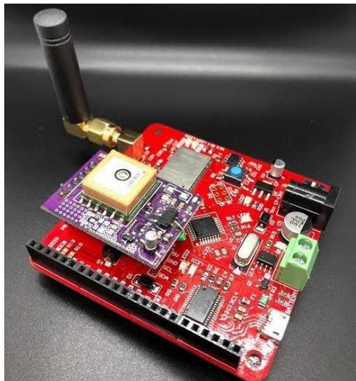
**Figura 7. Tarjeta embebida ATMEGA-328 Sigfox RCZ2.**
