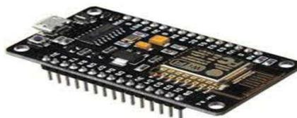
Figura 6: Tarjeta NodeMCU
