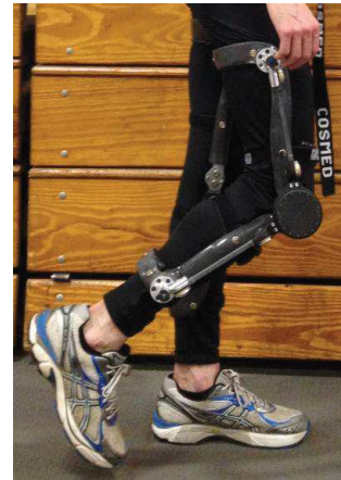
Fig. 5 Ejemplo de exoesqueleto para rodilla. Imagen de “G. Elliott, G. S. Sawicki, A. Marecki and H. Herr. The biomechanics and energetics of human running using an elastic knee exoskeleton , IEEE 13th International Conference on Rehabilitation Robotics (ICORR), Seattle, WA, 2013, pp. 1-6.”
