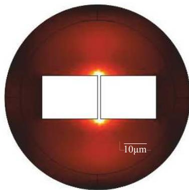
Fig. 2. Classical dipole geometry revealing less electromagnetic field concentration.
