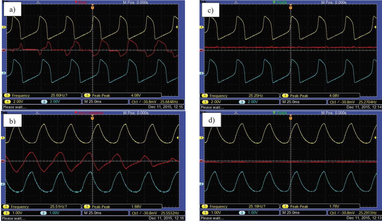
Figure 7: Experimental acquisitions of the PCB design. Without coupling:  $x_1$  and  $x_2$  in a) and  $y_1$  and  $y_2$  in b). With the coupling from Figure 5:  $x_1$  and  $x_2$  in c) and  $y_1$  and  $y_2$  in d).
