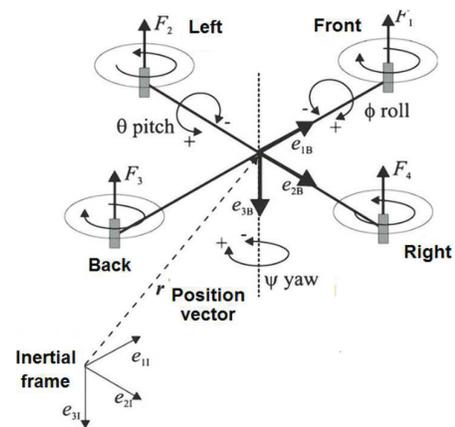
Fig. 1. Basic movements of a quadcopter.
