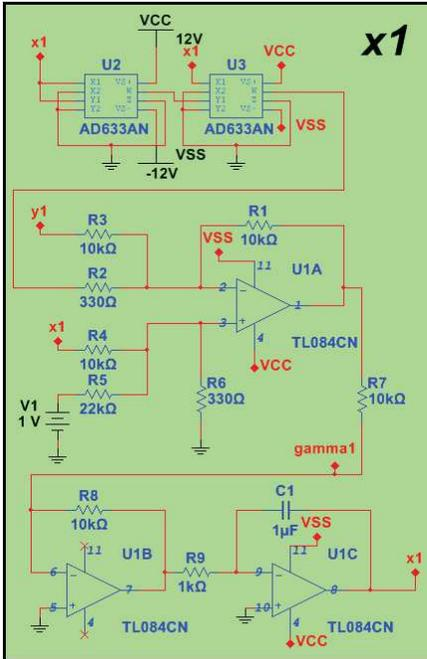
Figure 1: Schematic diagram of the  $x_1$  state given by (1).
