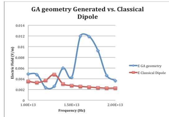
Fig. 6. Electromagnetic field collected by nanostructures. Line blue represents the GA generated geometry. Line red represents the rectangular classical geometry.
