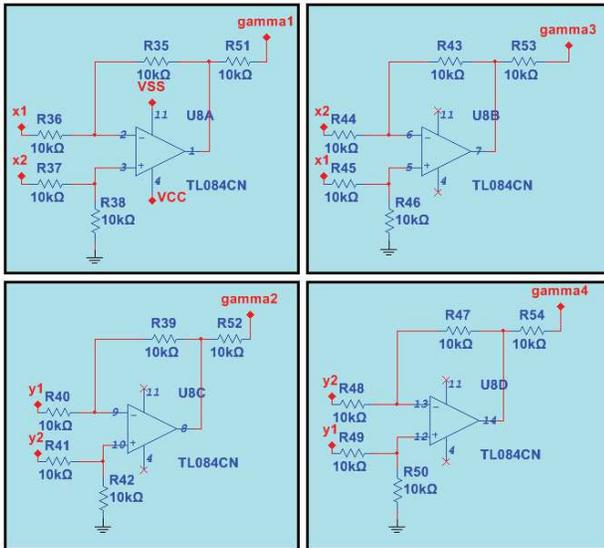
Figure 5: Schematic diagram of the  $\gamma$  coupling.
