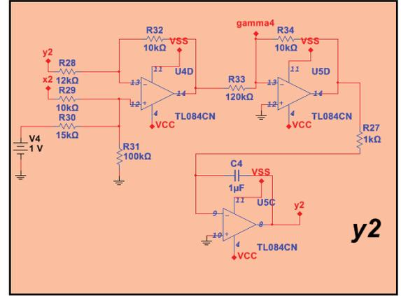
Figure 4: Schematic diagram of the  $y_2$  state of system 2.
