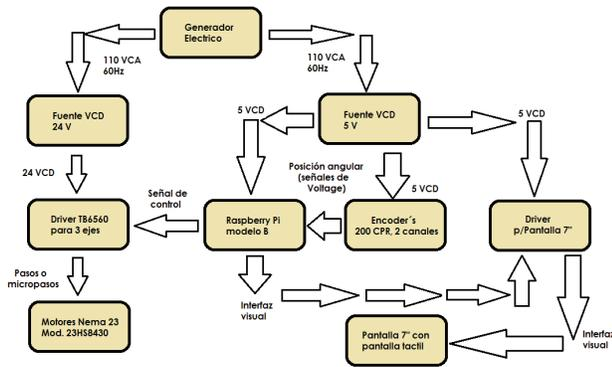
Fig. 5. Block diagram of electrical system
