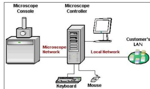
Fig. 3. Inspect F50 Scanning Electron Microscope schematic.
