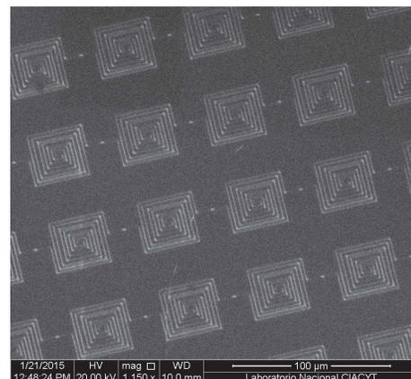
Fig. 8. Actual example of a nanostructure manufactured with the CAM module.
