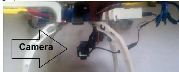
Fig. 9 Mounted camera on the quadcopter.
