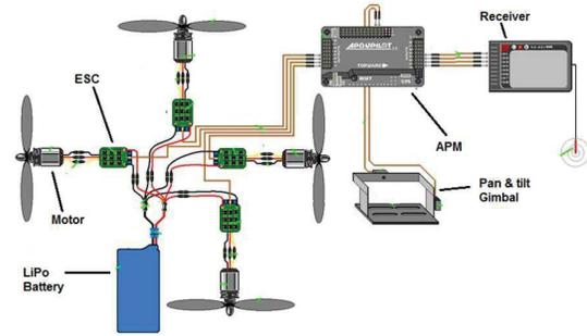
Fig. 8. Electric connections
