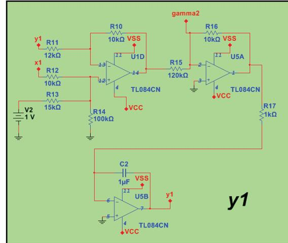
Figure 2: Schematic diagram of the  $y_1$  state given by (1).
