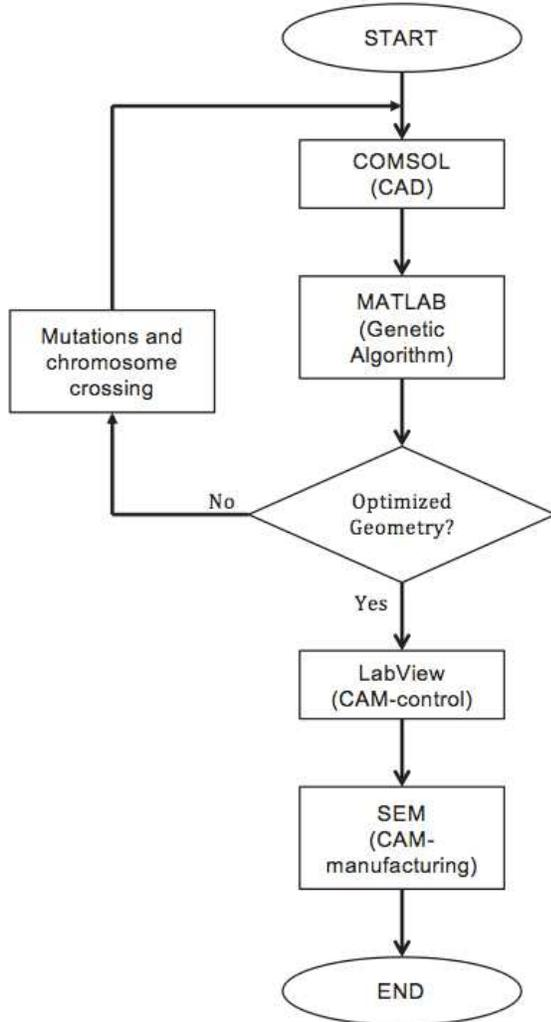
Fig. 5. CAD/CAM module flowchart.
