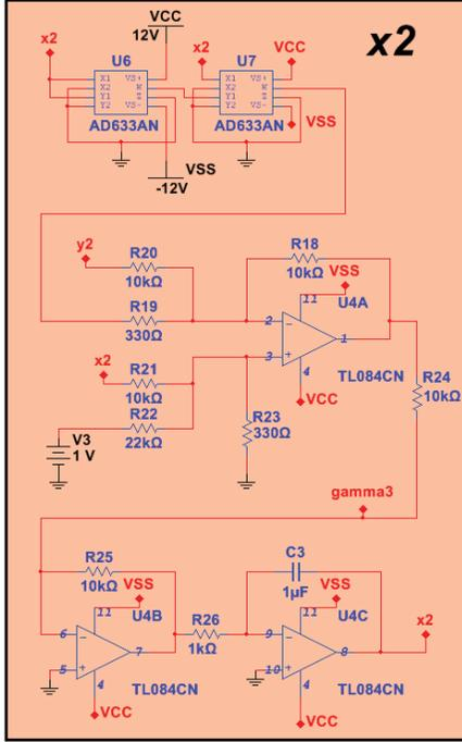
Figure 3: Schematic diagram of the  $x_2$  state of system 2.
