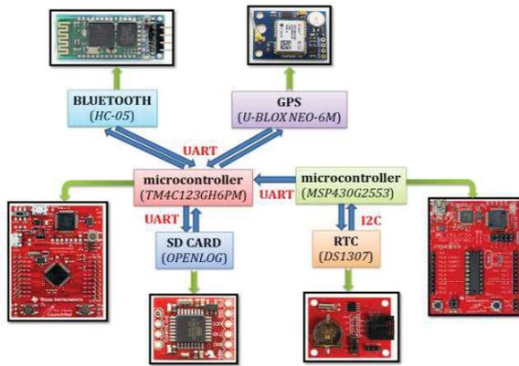
Fig. 1. Block diagram of the electronic system developed.
