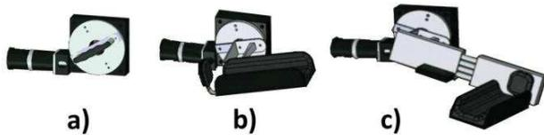
Fig. 4. Accessories of the mechatronic device for arm rehabilitation. a) wrist, b) Elbow, and c) shoulder.
