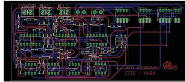
Figure 6: PCB design of the system given in eq. (4).
