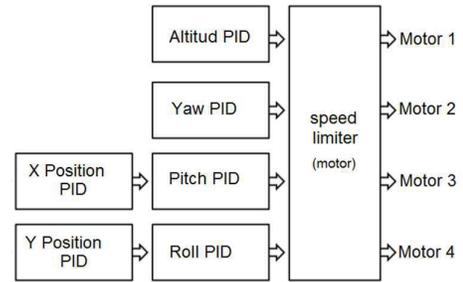
Fig. 3. Description of a quadcopter control.
