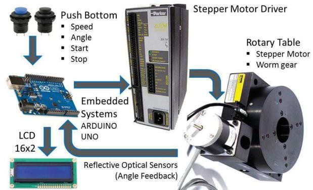
Fig. 2. Schematic diagram of mechatronic system
