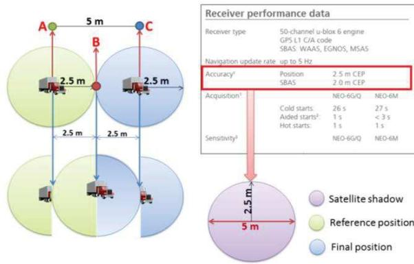
Fig. 2. Horizontal accuracy of the UBlox Neo 6m GPS module.
