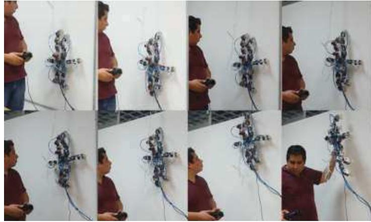
Figure 24. Vertical walking of WALL-BOT while is doing a visual inspection [8].
