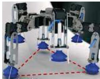
Figure 3. Hex-piderix robot: Stability polygon [6].
