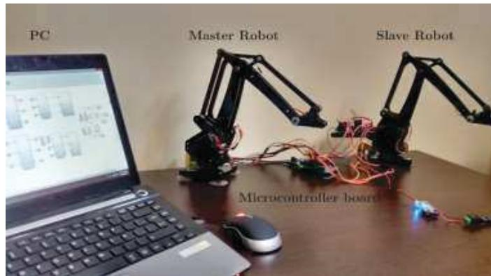
Figure 1. Experimental Platform. Consists of two Robot Manipulators, an Arduino Due board and a PC with MATLAB/Simulink®.
